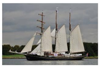
The "Gulden leeuw" (Golden Lion) has been designed and built as an ocean-going, 'A' class ship. In combination with the three-mast topsail schooner rig, it is a fast, robust ship. 70 meters long with 40 meter masts The Gulden Leeuw was originally built in 1937 and completely redesigned and rebuilt in 2010, the ship has preserved its 1930s heritage ambience, but offers practical use of space with a giant dormitory sleeping up to 60 trainee crew.
